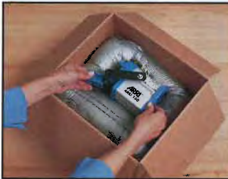
3. Place the expanding foam-filled bag in the shipping carton and nestle the product onto the cushion.
